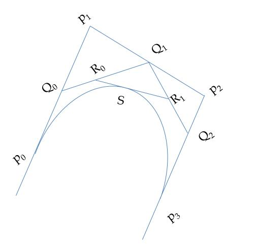
$p_{0}, p_{1}, p_{2}, p_{3}$  are fixed points  $Q_{0} = (1-t)p_{0}+tp_{1}$   $Q_{1} = (1-t)p_{1}+tp_{2}$   $Q_{2} = (1-t)p_{2} + tp_{3}$   $R_{0} = (1-t)Q_{0} + tQ_{1}$   $R_{1} = (1-t)Q_{0} + tQ_{2}$  $S = (1-t)R_{0} + tR_{1}$
