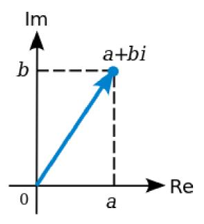
A complex number can be visually represented as a pair of numbers (a, b) forming a vector on a diagram called an Argand diagram, representing the complex plane. "Re" is the real axis, "Im" is the imaginary axis, and i is the imaginary unit which satisfies i2 = -1.
