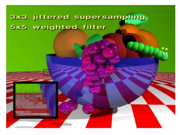
Each sample is perturbed by a random amount in x and y. The random amount is constrained to be less than one sixth of the pixel's width.
